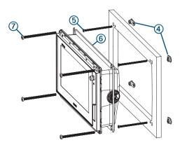
17 Secure the nut plates to the mounting surface by fastening the smaller machine screws (5) through the smaller holes.
